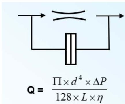
However, the pressure drop is extremely small (7 Pa maximum compared to the test pressure 100 000 Pa). So if a leak between two cavities is 200 sccm at 1 bar (100,000 Pa), if we take a linear approximation, the same leak under 7 Pa (worse case scenario) will flow  $200 \times 7 / 100000 = 0.014$  sccm.
