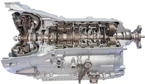
This casting process is prone to porosity, and with all these channels, the chances of an outer leak of fluid or an internal leak increase.
