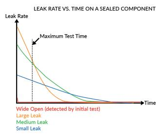
There is no time to wait for the perfect repeatable measurement: the faster the better. The goal is to stay in that area defined on the left side of the maximum test time on the diagram.
