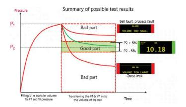
**Second, a regular pressure decay test** is performed if the watch passes the initial "large leak" test.
