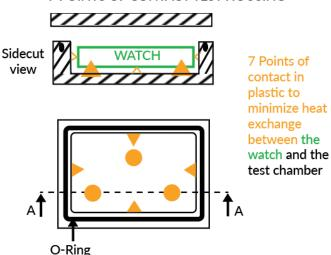
**Environmental Conditions.** It is always advisable to put heat insulation and reflective tape on the outside of the test fixture and test hoses. The test environment can heat up or cool down the test station, despite insulation.
